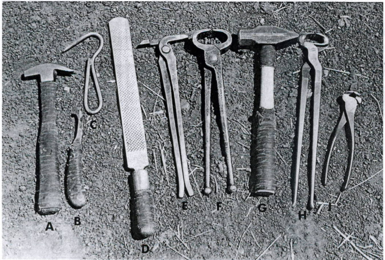
Tools: A) shoeing hammer, B) hoof knife, C) hoof pick, D) horseshoer's rasp, E) shoe spreader, F) pincers, G) anvil hammer, H) hoof nippers, and I) nail cutters.
