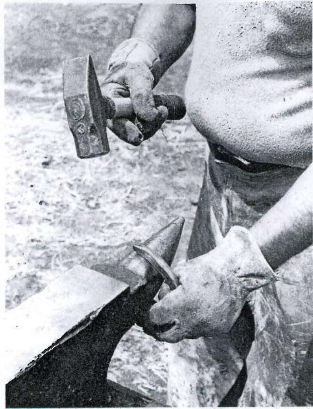
Shape shoe with anvil and hammer.
